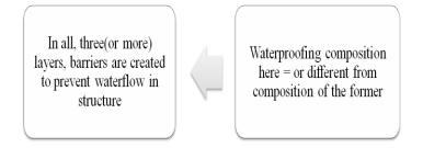
For binding the various layers, many types of reinforcement agents/ materials are used (eg polymers because of their inert nature). Also various waterproofing composition require a SOLVENT for making a waterproofing solution, which react with the SUBSTRATE.
