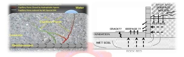
Up thrust action and buoyancy in contours against retaining wall, under reinforced basement flooring and underground basement spaces.
