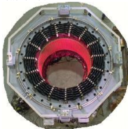
(1b.cross section of Powerformer stator)
