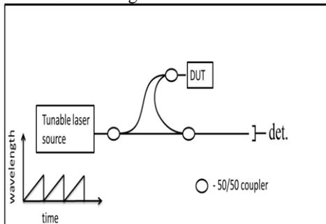
**Fig 1. Optical fiber network to measure Rayleigh backscatter signal of (FUT) [5].**
