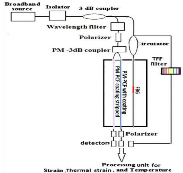
**Fig. 2 Schematic of the hybrid polarimetric-FBG sensor system.**
