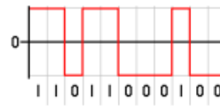
Fig-5 Bipolar NRZ format
