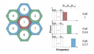
Figure. 1.2. FFR scheme[8]. In FFR, the reuse factor for interior users is 1 and the reuse factor for exterior users is 3.
