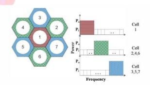
Figure 1..3. SFR scheme[6]. In this scheme inner RBs transmit with a higher transmit power than RBs used for cell-edge users.
