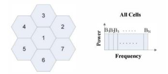
Figure.1.1. Reuse-1 scheme deployment[6]. In this scheme all the cells transmit on all available sub-carriers in the spectrum with the same power
