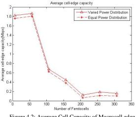
Figure 4.2: Average Cell Capacity of Macrocell edge users
