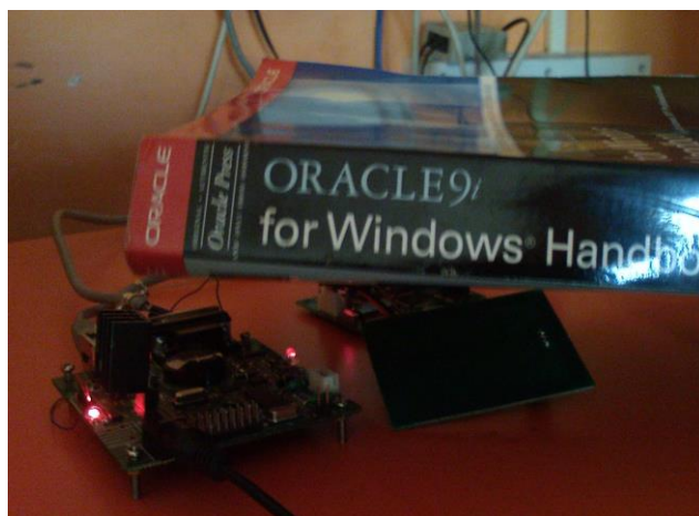
Figure 7: Tagged book showing to the antenna
