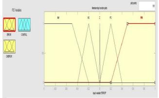
Fig.7:Membership function for input (error)
