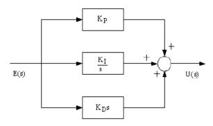
Fig 2: PID controller system block diagram.
