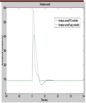
Fig.15:Armature current characteristics of dc motor using fuzzy and PID controller
