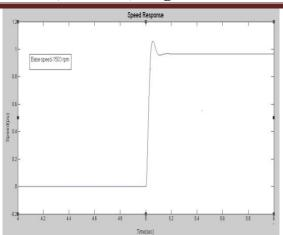
Fig.11:Step responseof dc motor with PID controller
