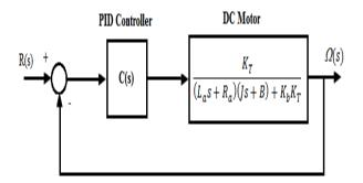
Fig. 3: PID DC motor speed control system block diagram
