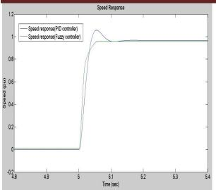
Fig.13:Comparison of speed response of dc motor using fuzzy controller and PID controller
