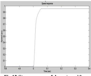
Fig.12:Step response of dc motor with PID controller
