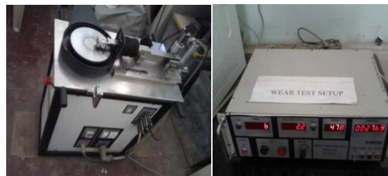
Fig 1: Set up to Perform an Abrasive Wear Test on Pin-on-Disc
